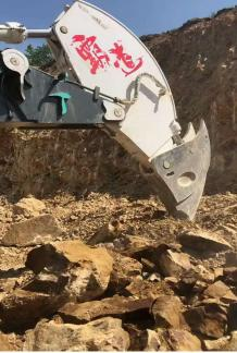
The J-shaped hooking and prying rock boom combines the advantages of the traditional rock boom and the integrated arm and ripper, and retains the advantage of the integrated arm's digging depth. Adding the ripper cylinder makes the entire forearm and ripper more flexible and can adapt to most working conditions.
